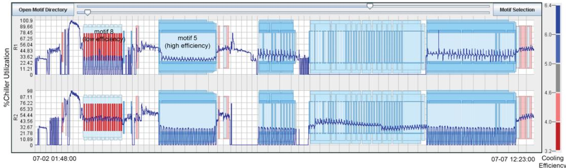
Figure 1: Frequent Patterns (Motifs) Discovered in Data Center Chiller Time Series
