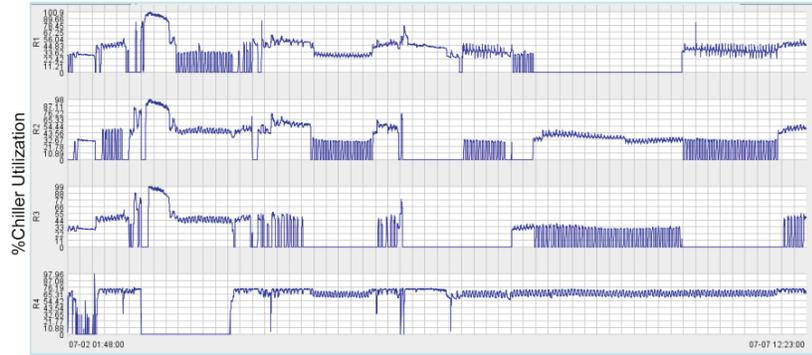
Figure 11: Data Center Chiller (R1-R4) % utilization regular time series without motif
