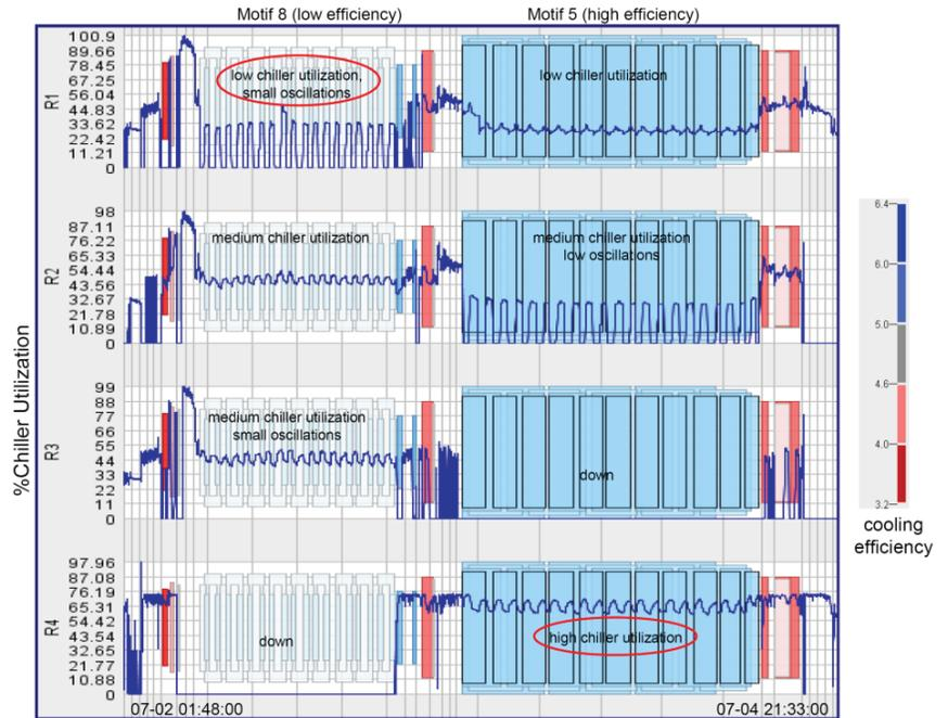
Figure 8: Motifs 5 and 8 are Enlarged to Compare their Chiller Utilization. Motif 5 is more efficient than motif 8. Motif 8's chillers R1 and R3 have some oscillatory behavior. (x-axis: 07-02 01:48 to 07-04 21:33, y-axis: %utilization of chillers R1-R4, color: cooling efficiency).
