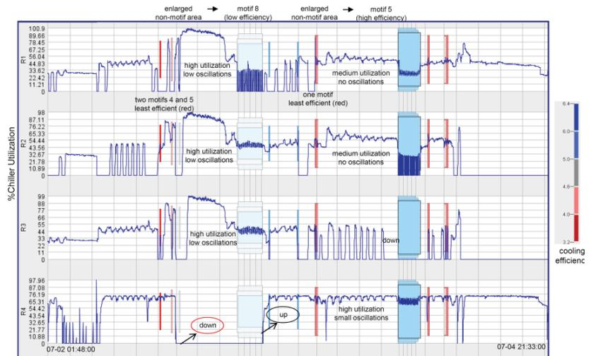
Figure 9: Enlarge the non-motif area to observe the transitions from low cooling efficiency motif 8 to high cooling efficiency motif 5. (x-axis: time line from 07-02 01:48 to 07-04 21:33, y-axis: %utilization, color: cooling efficiency).
